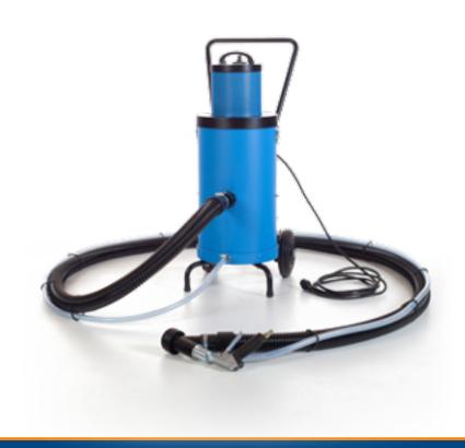
This compact electric-pneumatic driven injection vacuum blasting machine with an average blasting pattern of 16 mm width, is excellent to apply for blast cleaning weld seams, spot blasting of smaller areas, inspection and repair of engines and machinery overhaul, bodywork on vehicles.
