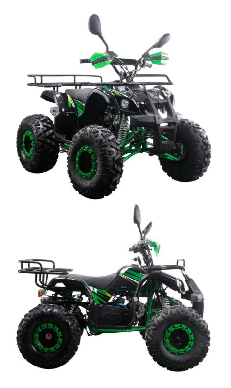
110cc or 125cc engine, 4-stroke,air cooled full automatic (reverse gear available) electric start
