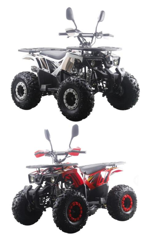
110cc or 125cc engine, 4-stroke,air cooled reverse gear electric start
