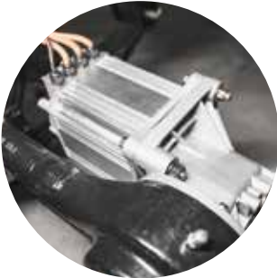
4 kw permanent magnet synchronous motor
