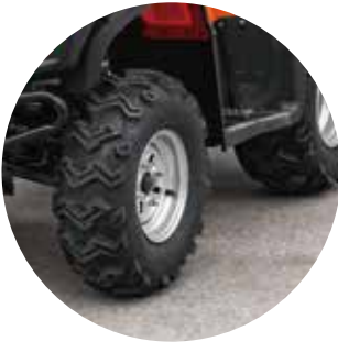
22-inch W-shaped off-road tire + iron hub combination
