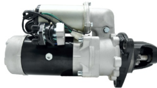
Models: PC360-7 Engine: 6D114 Power/voltage: 11A/24V
