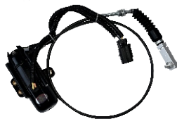
CAT305-307 throttle motor Applicable model:E305E/E307E
